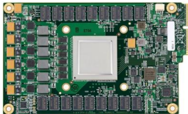
Google's Tensor Processing Unit, an Inference Data Center Accelerator
