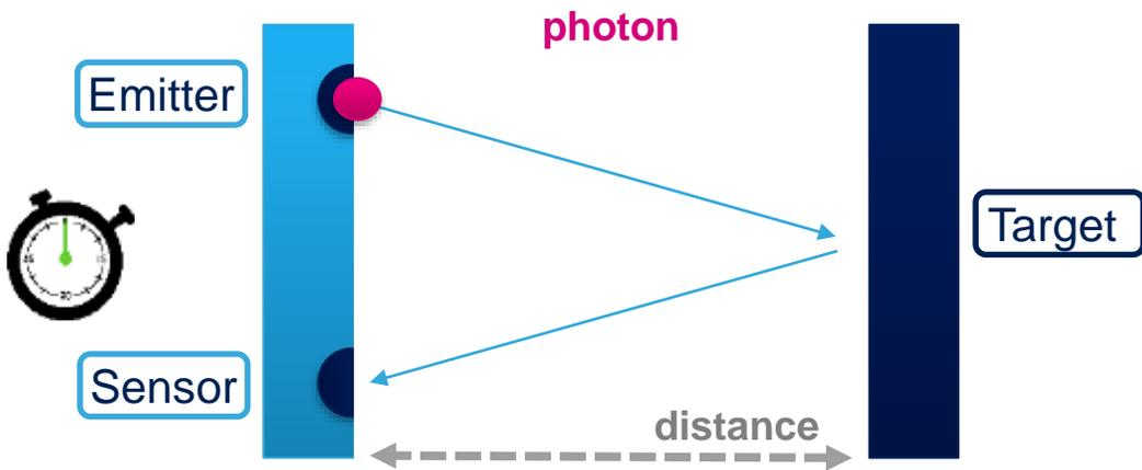
$$\text{Measured distance} = \text{Photon travel time} / 2 \times \text{Speed of light}$$
